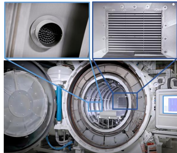
Figure 12. Test furnace with next generation of PLANSEE refractory metal hotzone equipped with “flowbox” and gas nozzle inserts [11].
