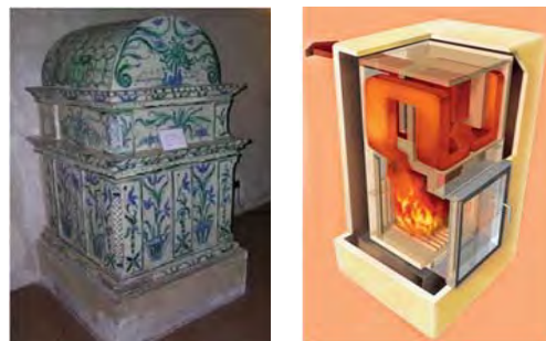
Figure 1: Left: historical “Sfruz” heat accumulation stove, located in the Buonconsiglio Castle in Trento, Italy. Right: view of a project design of a modern stove, where combustion chamber and twisted conduit are visible.
