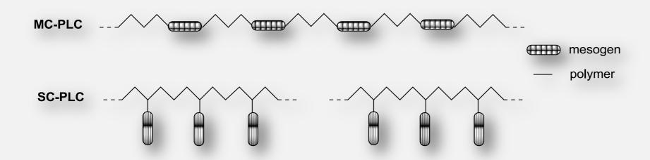
LCE are a particular kind of PLC [1]. Are rubber-like materials which react to external stimuli [2], depending on the orientation of the molecules, the absorption coefficient of the medium and the light intensity.
