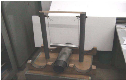
Figure 12. Experimental setup for LISS tube measurement
