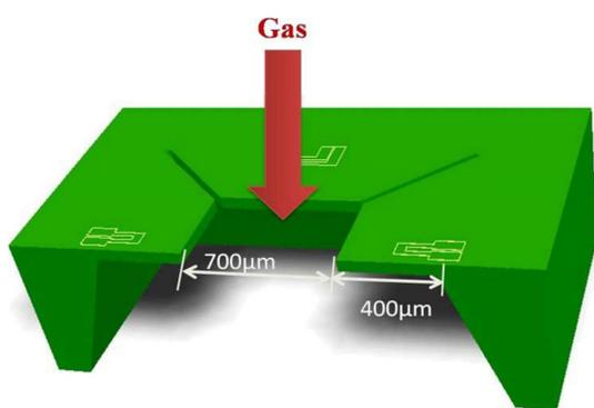
Figure 1. Schematic diagram of flow sensor.
