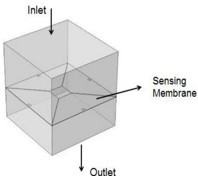
Figure 2. Geometry of Flow Pressure Sensor
