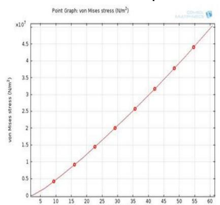
Figure 6. Stress vs. pressure (Gasoline)
