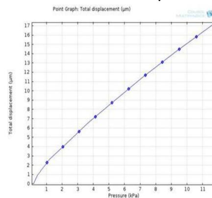
Figure 5. Displacement vs. pressure (Gasoline)
