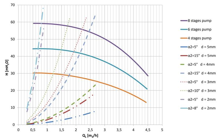
Figure 3. Pump and ejector characteristic curves
