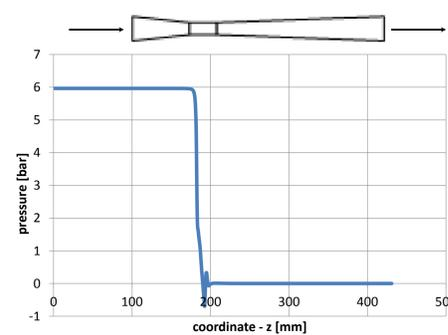
Figure 4. Pressure trend along the ejector
