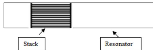
Schematic of 2D linear thermoacoustic wave generator
