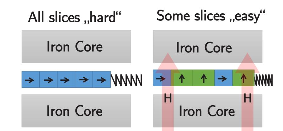
The MSM Element in the actuator is divided in several individual areas. These areas are also called slices. The magnetic characteristic of each slice is anisotropic and therefore each slice has a defined magnetic orientation which is divided in "hard" (blue) and "easy" axis (green).
