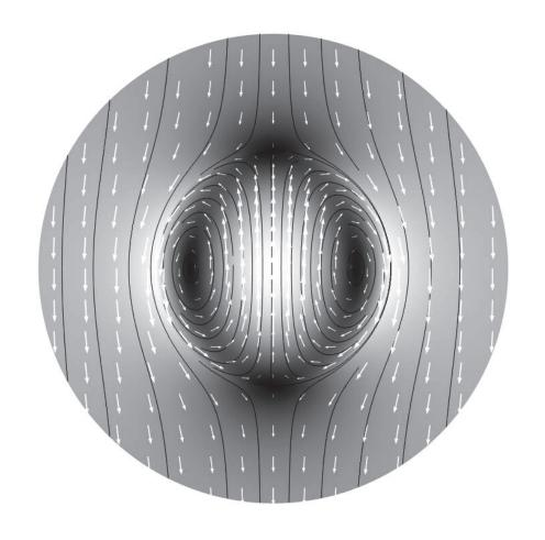
Velocity in a plane containing the axis of symmetry: shading shows fluid speed; solid lines show streamlines; and arrows show velocity vectors.
