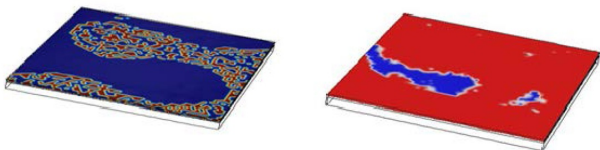
Figure 2: Contact area and plastic zone.
