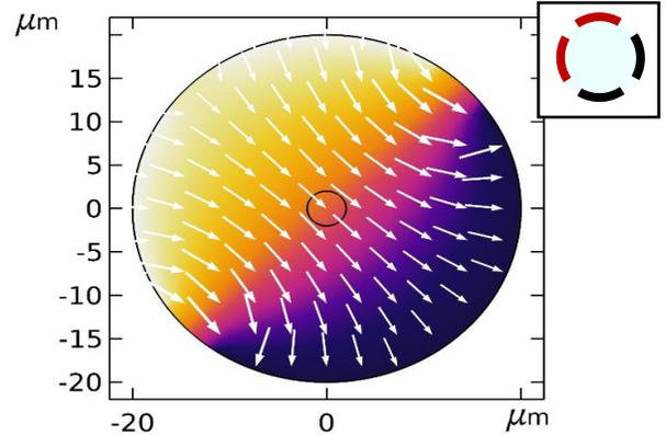
**Figure 3:** Applied electric field distribution along a cross-section of the EOPM with both electrodes active and (inset) corresponding electrode map using the format depicted in Figure 1.
