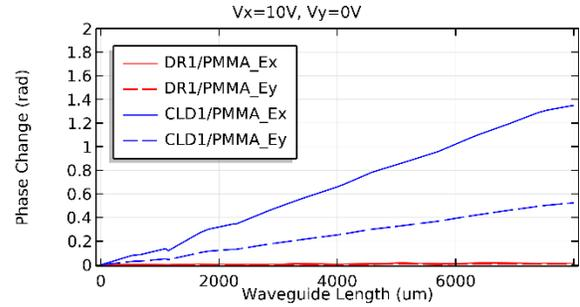
**Figure 5:** Phase shift in propagating X-polarized light ( $E_x$ ) as a function of waveguide length when only the X-axis electrode is active, and corresponding static phase shift induced in orthogonally polarized ( $E_y$ ) light.
