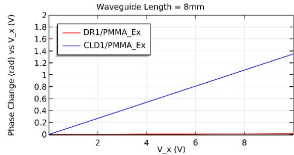
**Figure 6:** Phase change as a function of applied voltage along the X-axis.
