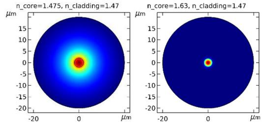
**Figure 4:** Fundamental mode profiles for CL1/PMMA (left) and DR1/PMMA (right).
