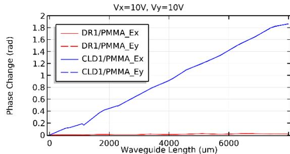
**Figure 7:** Phase change as a function of waveguide length when both electrodes are active.
