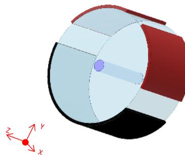
**Figure 2:** Three-dimensional view of proposed configuration for dual polarization modulation. The signal electrodes are represented in red and ground electrode in black. As both ground electrodes are electrically equivalent, they are considered to be a single electrode so as to reduce fabrication complexity. The EOP core is shown in blue, and surrounded by concentric glass cladding.
