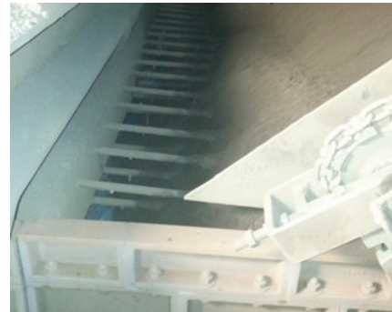
Figure 3. Sinter plant feeding system in operation with two rows of horizontal permeability bars.
