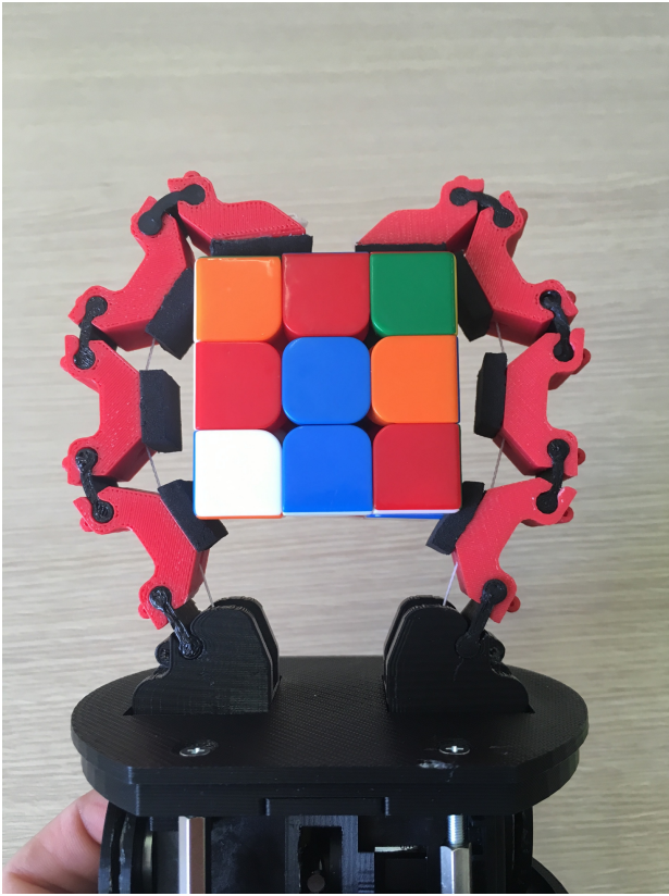
Figure 1: A modular underactuated gripper grasping a cubic object. In this example passive joints were designed in order that finger tips reproduce a given trajectory.
