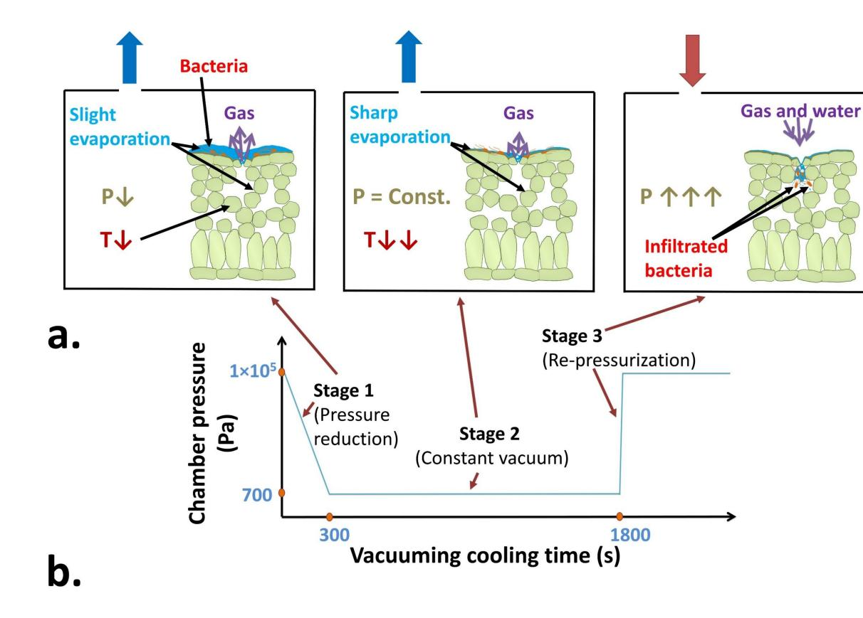
**COMPUTATIONAL METHODS**: We developed a mechanistic multiphase transport model to simulate passive infiltration of pathogenic bacteria (initially being in a liquid film at the leaf surface) into a spinach leaf through one stomate during the vacuum cooling process.
