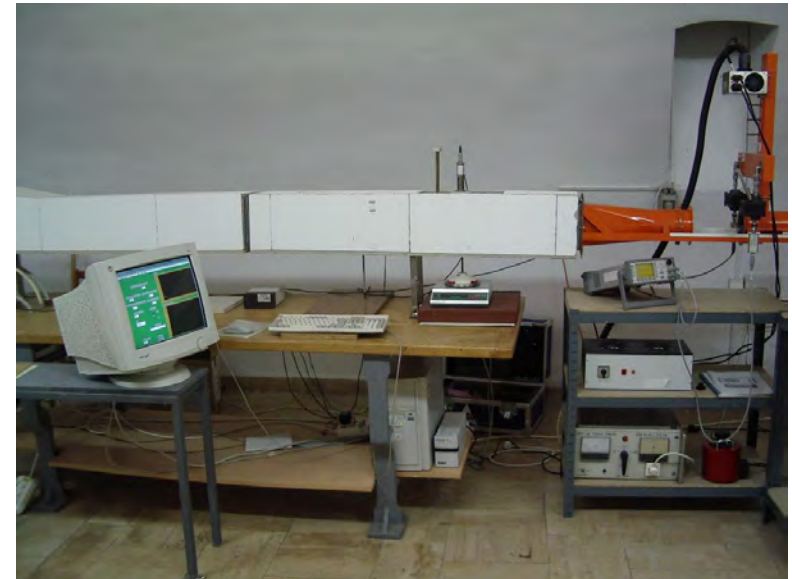
Experimental convective drying tunnel
