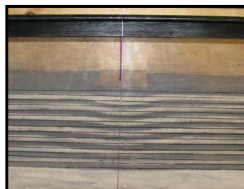
Figure 2: Shear failure in Philippi Dune sand [1]
