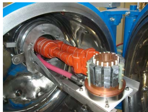
Figure 3. Crucible of the CCIM installation at University of Mondragon.
