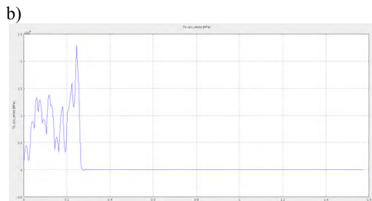
Figure 23. Contact pressure progress vs slave boundary arc length for h_{max}=35.2\mu\text{m} . a) Ideal tip; b) Truncated tip.
