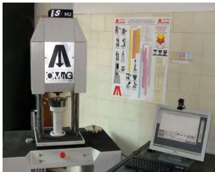
Figure 12. Universal Hardness Testing Machine OMAG SR-HU 09 produced by Omag Affri S.p.a.
