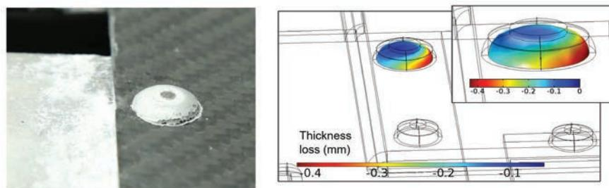
**FIGURE 7.** Time-dependent analysis (right) used to determine the dissolution of the aluminum rivet (left).
