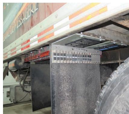
**FIGURE 2.** Top: Galvanic corrosion damage induced on a multimaterial overlap assembly made of a carbon-fiber-reinforced polymer (CFRP) and a 6000 series aluminum alloy after one year of in-service exposure on a vehicle. Bottom: Typical mounting of samples on a vehicle for in-service exposure testing.
