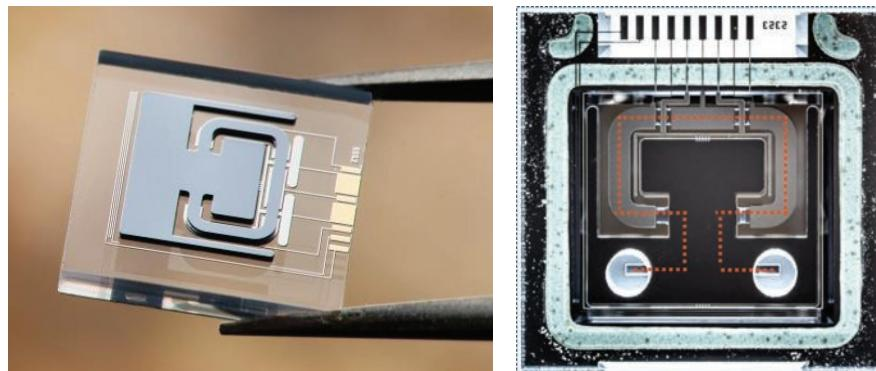
**FIGURE 4.** MEMS Coriolis chip used for density and viscosity measurements. Left: Complete sensor held by pliers. Right: Chip layout inside the device.
