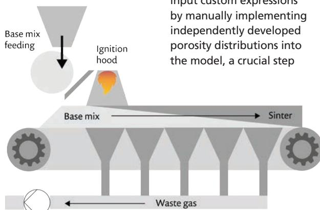
FIGURE 1. Sintering process scheme.
