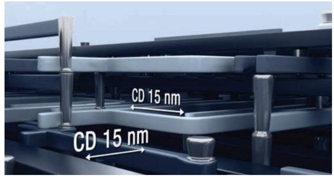
**FIGURE 1.** The critical dimensions inside a smartphone processor measures in nanometers. To put it in perspective, a human hair measures 5300 times larger than the critical dimensions in these chips.
